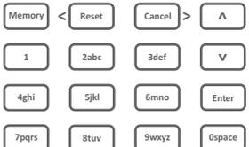
Using the Keypad enter the GSM number that will receive a SMS. Press the RESET button for 2sec to clear the blocks if you make an error or to try and clear a zero to type a calling code like +27\_.
